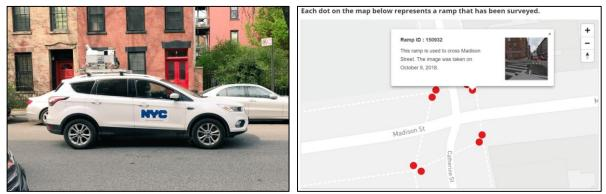
This survey utilized mobile technology to capture high definition, street level imagery and ground-based LiDAR data. The data was analyzed through an automated process to extract the measurements of each ramp. The survey locations and assessment results are available on the <u>Pedestrian Ramp Program Website</u>. There are a total of 217,678 ramps in the five boroughs.<sup>1</sup> A map of program progress is also available in the <u>Program Progress</u> section of the website.
