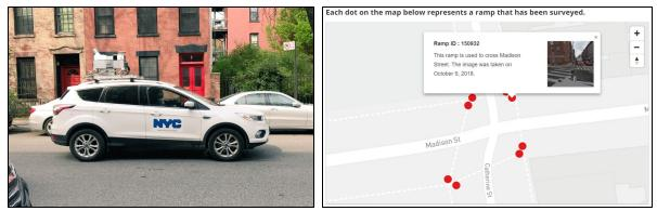
This collection utilized mobile technology to capture high definition, street level imagery and ground-based LiDAR data. The data was analyzed through an automated process to extract the measurements of each ramp. The locations and assessment results are available on the <u>Pedestrian Ramp Program Website</u>. There are a total of 217,678 ramps in the five boroughs.<sup>1</sup> A map of program progress is also available in the <u>Program Progress</u> section of the website.
