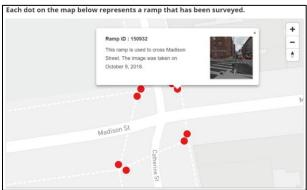
This collection utilized mobile technology to capture high definition, street level imagery and ground-based LiDAR data. The data was analyzed through an automated process to extract the measurements of each ramp. The locations and assessment results are available on the <u>Pedestrian Ramp Program Website</u>. There are a total of 217,678 ramps in the five boroughs.¹ A map of program progress is also available in the <u>Program Progress</u> section of the website.
